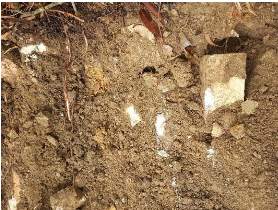
Fig 35 Photo of soil profile showing fill material with small tree roots < 20mm Ø
