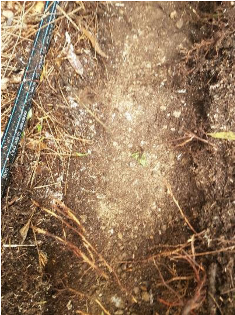
Fig 30. Photo of hard compacted layer of gravel and sand in trench 1
